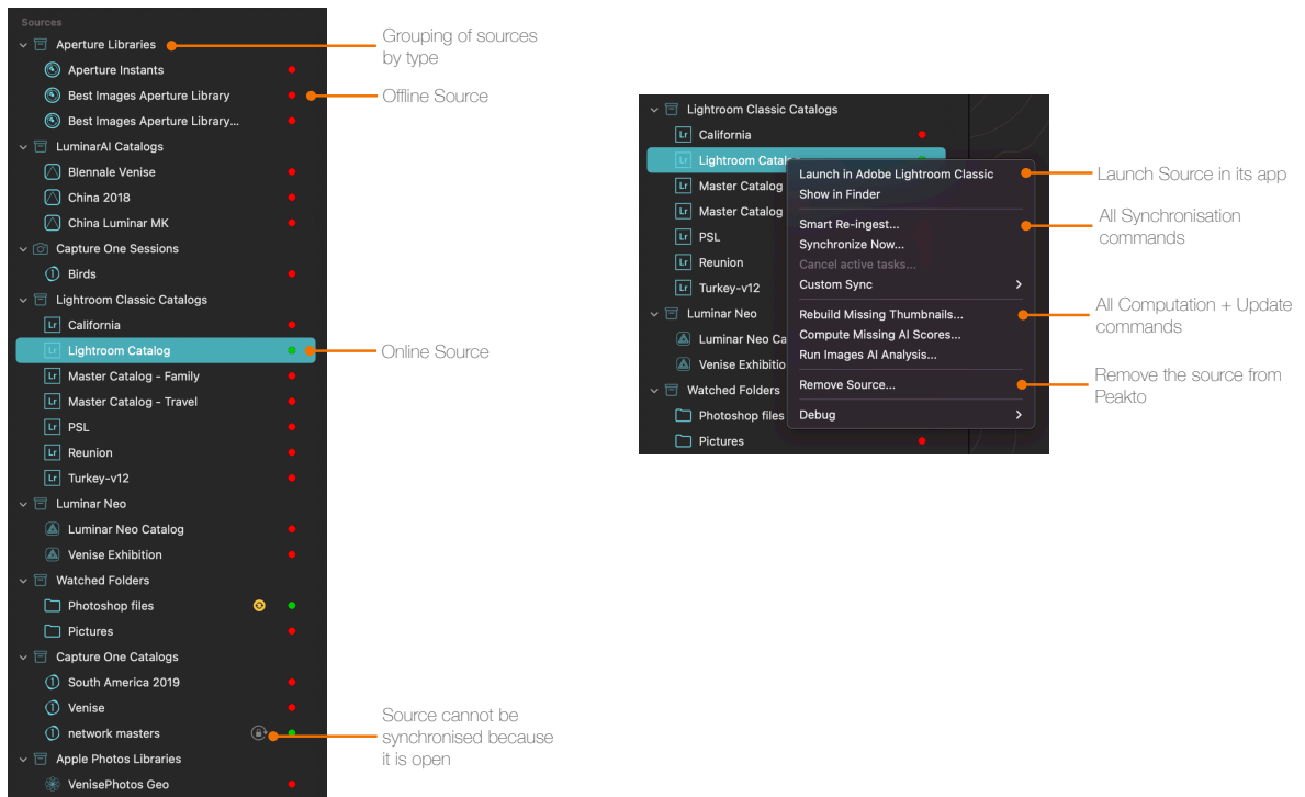
The sources in the sidebar (left). The contextual menu (right) that gives access to many possible actions on the source.
